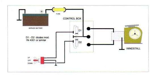
N Circuit - The central wire of the main switch is connected to the negative pole. The blanking of the overvoltage derives from the connection of the two diodes D1 and D2 to the control box as in the Figure above, i.e. with the reference lines (cathode) towards the central fastons.
