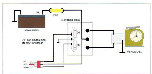
P Circuit - The central wire of the main switch is connected to the positive pole. The blanking of the overvoltage derives from the connection of the two diodes D1 and D2 to the control box as in the Figure above, i.e. with the reference lines (cathode) towards the lateral fastons.
