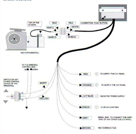
ACCORDING TO THE TYPE OF INSTALLED SYSTEM, THIS WIRE COULD BE CONNECTED TO THE POSITIVE OR NEGATIVE POLE.
