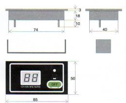
WHEN THE ANCHOR CHAIN IS IN ACTION, THE DISPLAY (S) AUTOMATICALLY STARTS TO WORK AND TO COUNT THE METERS OF CHAIN DESCENDING OR ASCENDING.
